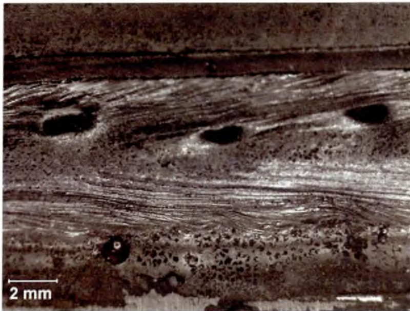
Figure 117. Photo showing surface breaking pores on a lap joint of LDX 2101 to Dogal 260RP-X with 309L-Si filler
