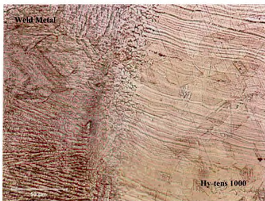
Figure 112. Hy-tens 1000 and Weld Metal Interface etched in 10% oxalic acid martensite in the HAZ and the weld material.
