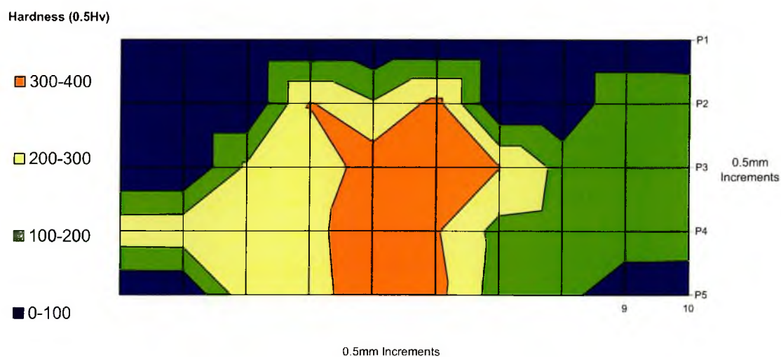
Figure 92. Series 7 microhardness map of fatigue sample 7.8.6, the sample failed the fatigue test at 8.0kN after 843525 cycles.
