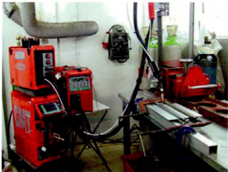
Figure 22. CMT Welding Equipment at Sheffield Hallam University.
