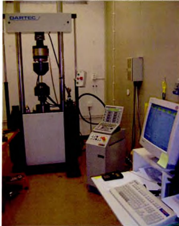
Figure 46. Dartec M1000/RK and Instron console 8500+ with software Cyclic version 17.7 at Outokumpu Avesta Research Centre, Avesta, Sweden
