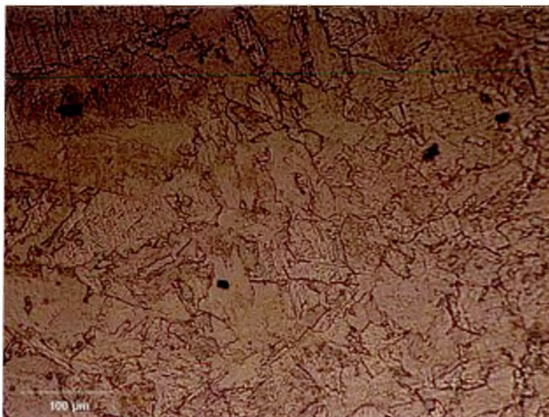
Figure 133. Typical Microstructure of Dogal 260RP-X HAZ in a CMT Dissimilar weld
