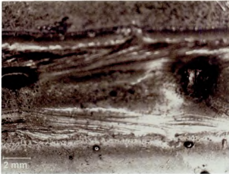
Figure 116. Photo showing surface breaking pores with cracking on a lap joint of Hy-Tens 1000 to Dogal 260RP-X with 309L-Si filler
