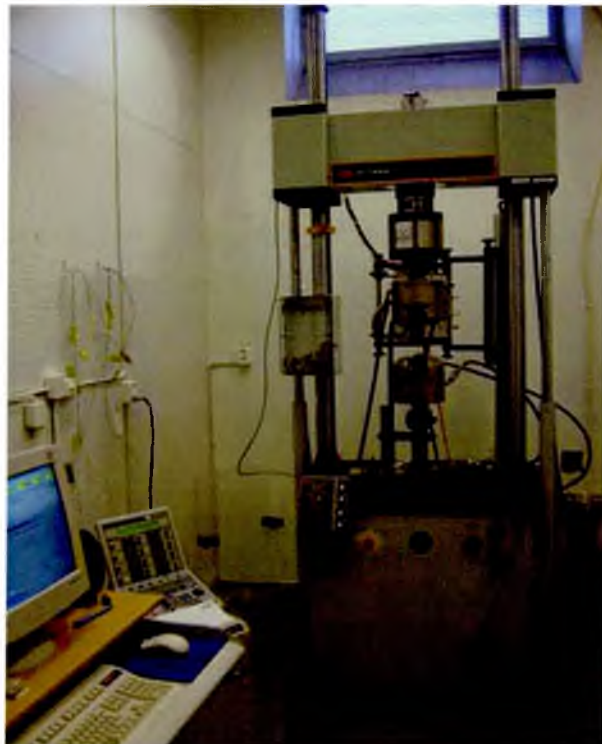
Figure 45. Instron 8502 and Instron console 8500+ with software Cyclic version 17.7 at Outokumpu Avesta Research Centre, Avesta, Sweden.
