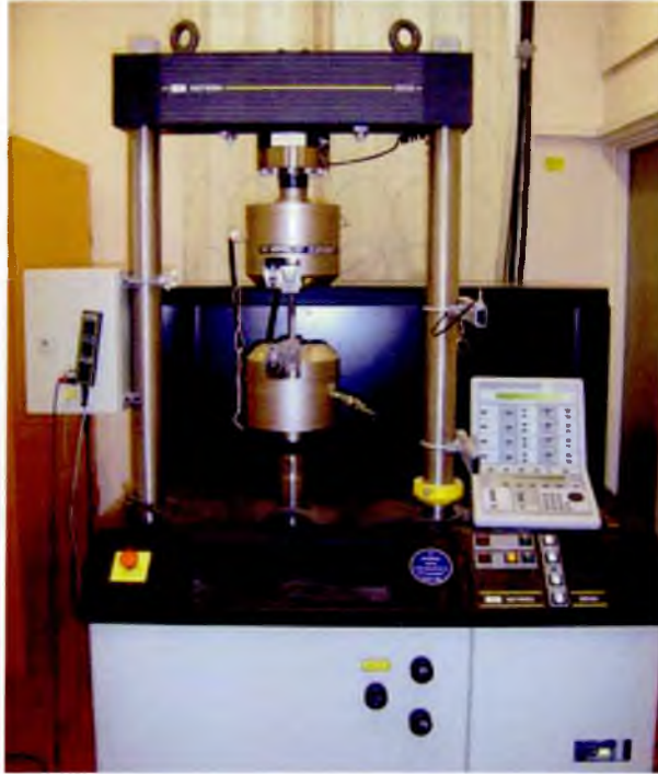
Figure 44. Instron 8516 and Instron console 8500+ with software Cyclic version 17.7 at Outokumpu Avesta Research Centre, Avesta, Sweden.
