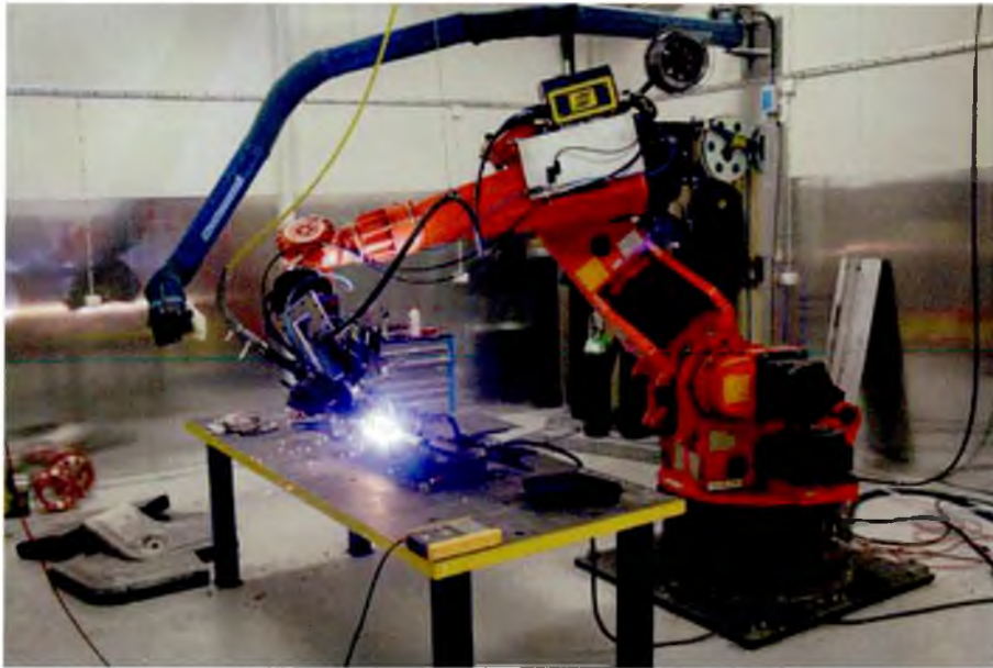
Figure 16. Laser Hybrid Welding Equipment at ESAB Process and Development Centre, Gothenburg, Sweden, April 2006.
