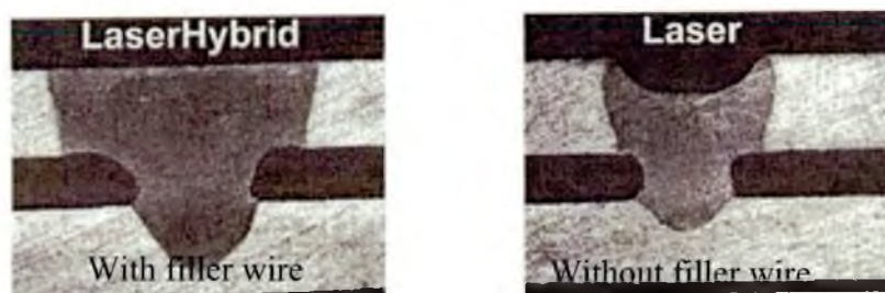
Figure 4. Effect of filler wire in the laser hybrid welding process when compared to that of laser welding 22
