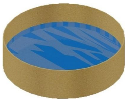
Step 1: PDMS was added to a paper cup, and cured.
