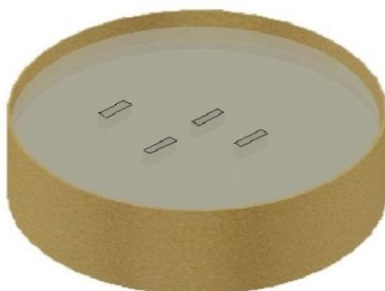
Step 3: After curing, Glass slides were removed to obtain Open-chambers.
