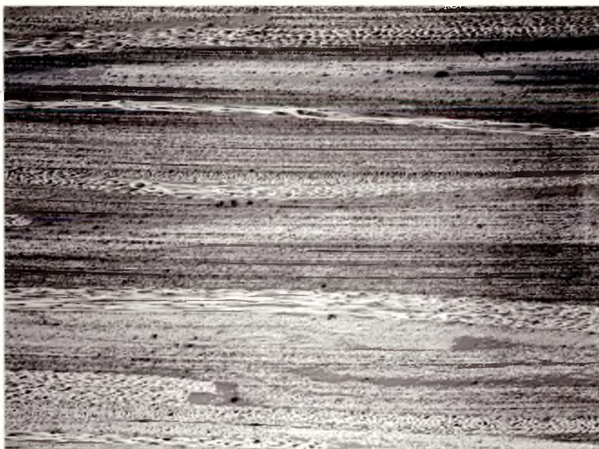
Figure 97 Side view of a polished 25.4mm sample. X20 Showing relatively few PEEK rich zones for this size of particle.
