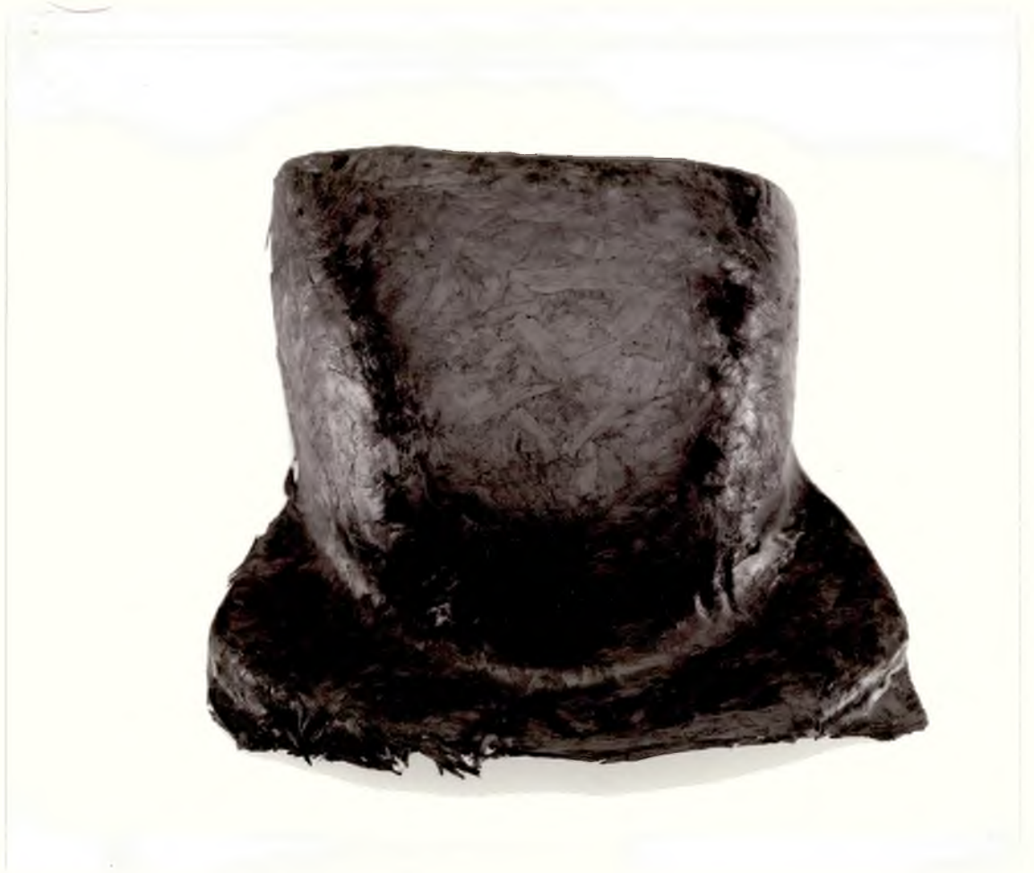
Figure 60 A moulding with a large radius of curvature containing Mono Munched particles, without tearing but slight wrinkling.
