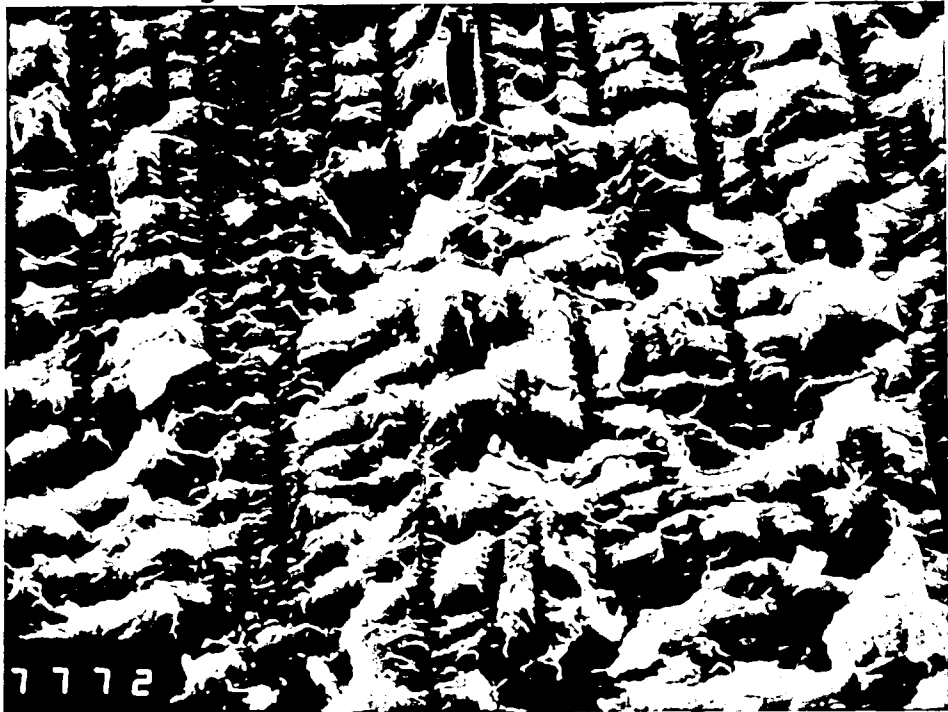
Figure 116 20μ X400 Higher magnification view of white region showing more massive deformation than the cleavage mode.
