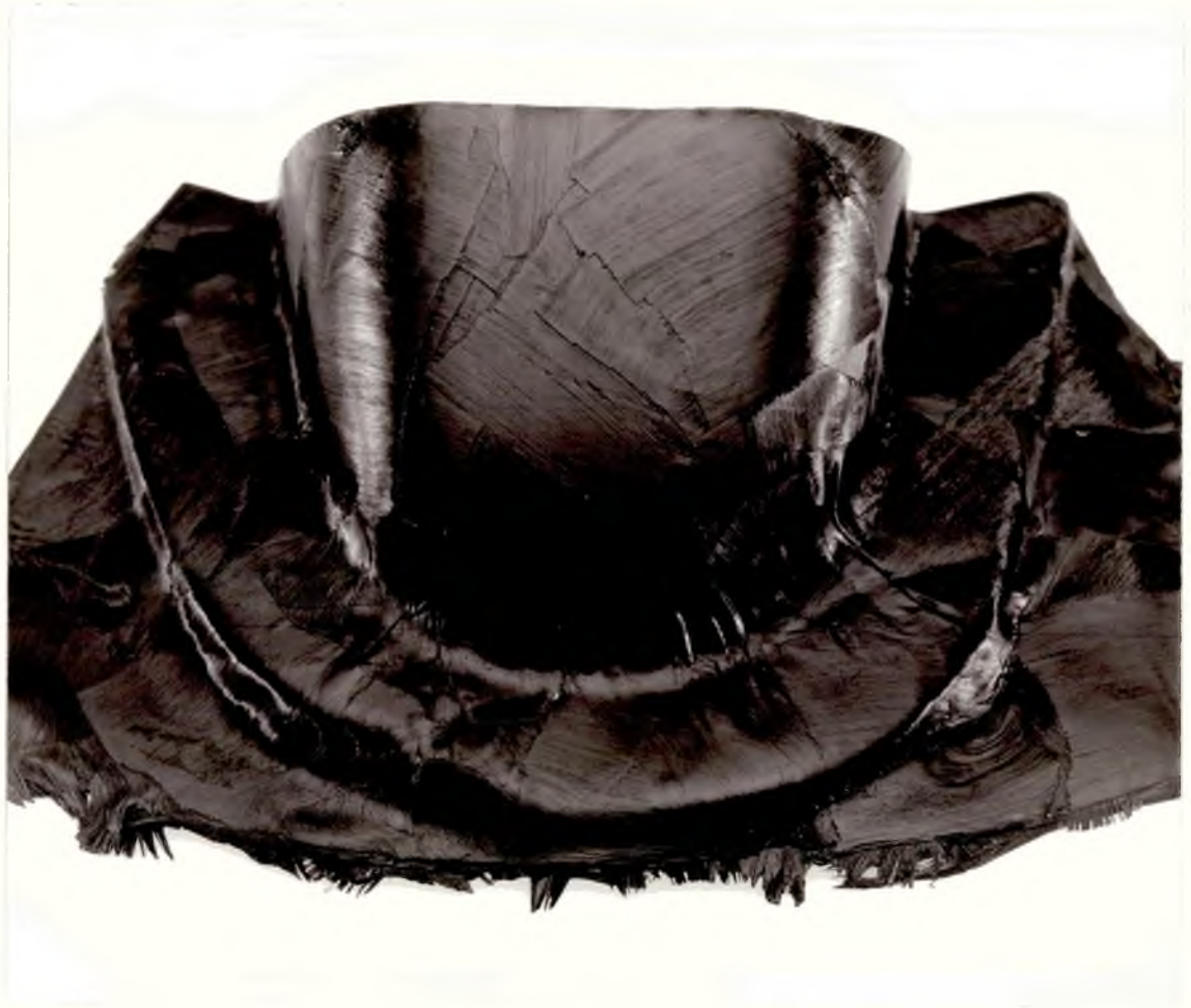
Figure 61 A moulding with a large radius of curvature containing 25·4mm square particles, without tearing but a large degree of wrinkling.
