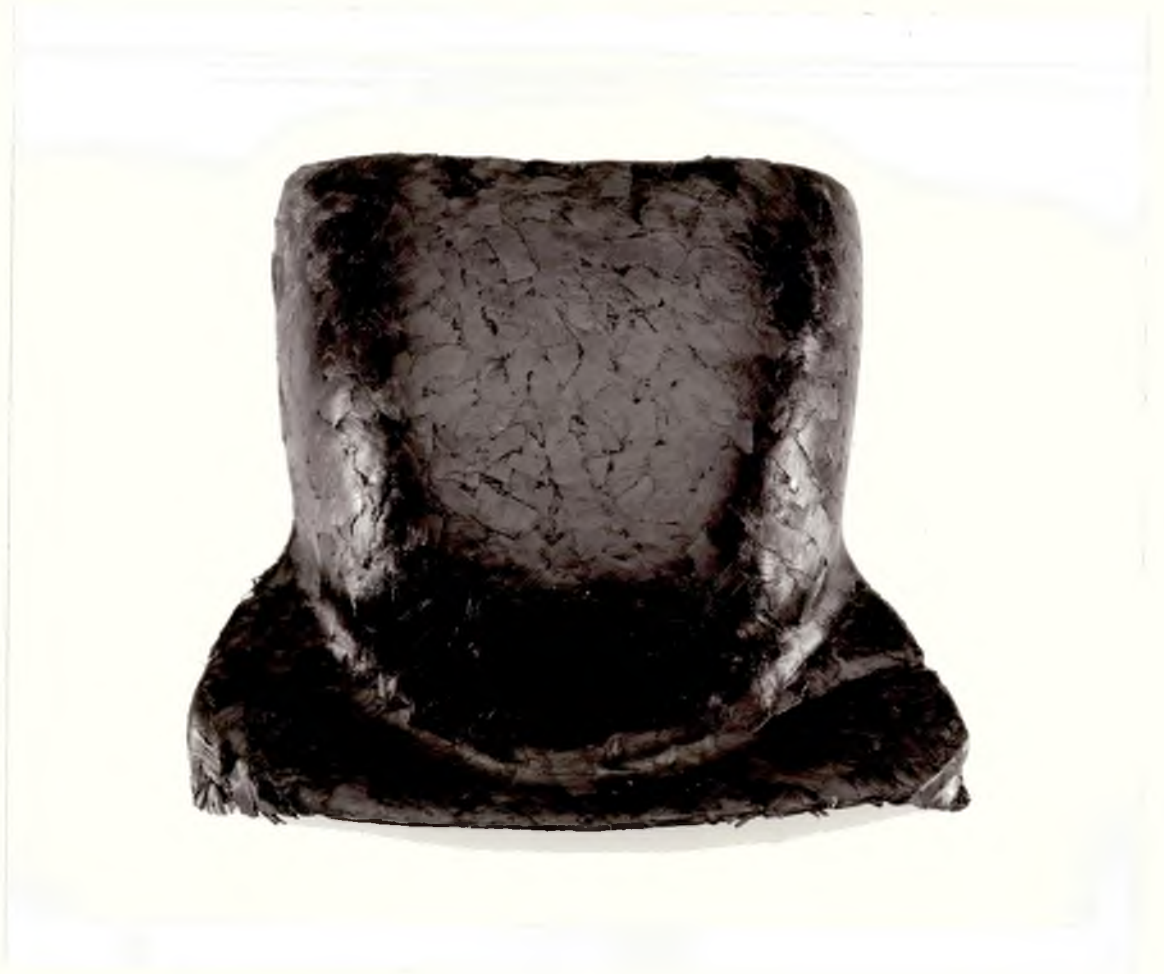
Figure 59 A moulding with a large radius of curvature containing 0.125mm square particles, without tearing or wrinkling.
