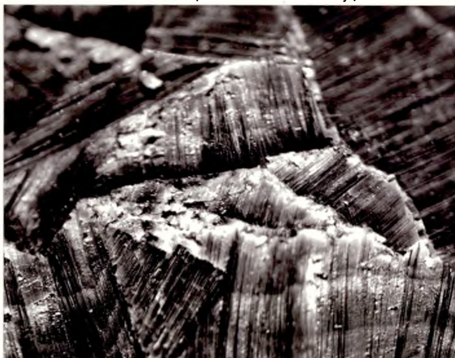
Figure 102 Oblique light micrograph of the fracture surface of a 6.35mm sample, X25 Several particles meeting with a central PEEK rich region.
