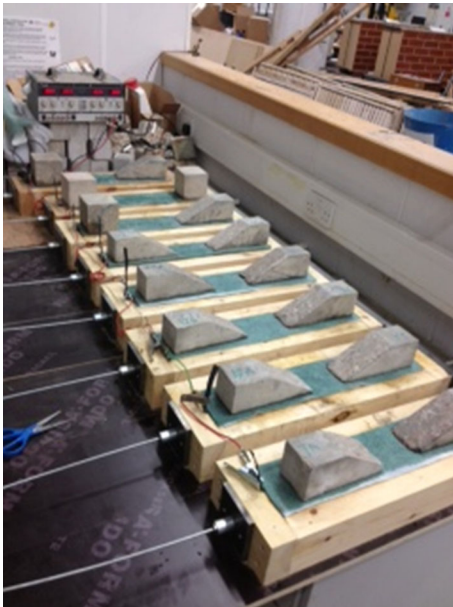
Fig. 2 Accelerated corrosion of tendons via power supply (top left)
