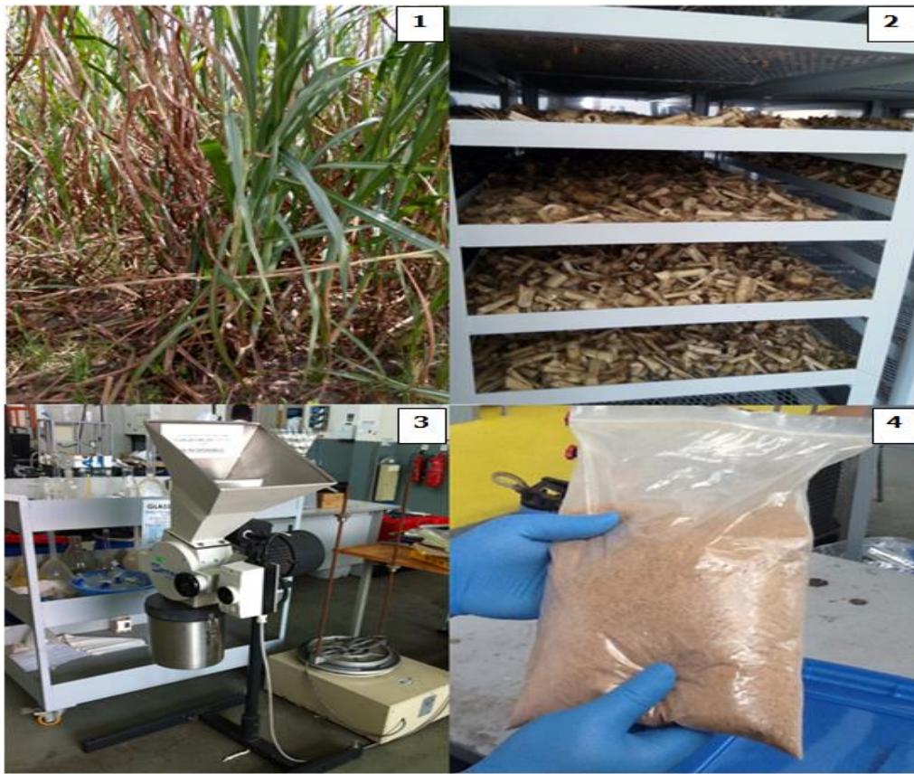
Figure 1: Pre-processing of Napier grass. (1) Napier grass on the field (2) chopped Napier grass stem (NGS) in the dryer (3) Rotor beater mill (4) Ground Napier grass biomass
