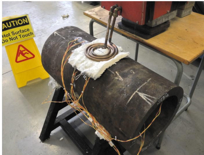
Figure 7. Induction heat treatment of the pipe after completion of the WeldCore® process.
