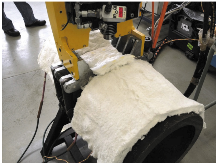
Figure 6. FTHP processing platform in-situ on a section of thick walled steam pipe. The pads are for preheating the pipe to approximately 200°C prior to commencing the WeldCore® process.
