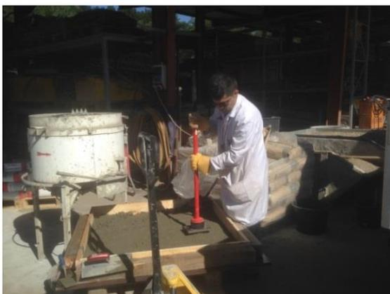
Figure 4. Compaction of newly cast mix.
