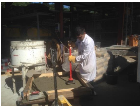
Figure 4. Compaction of newly cast mix.
