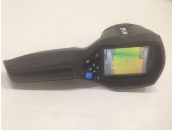
Figure 7. Thermal camera for monitoring the surface temperature of the slabs.
