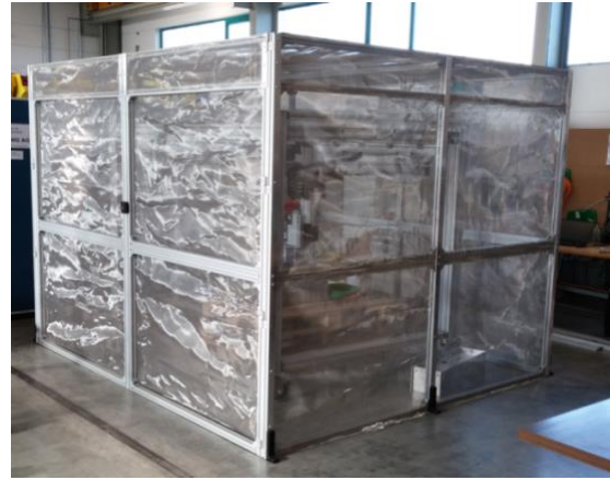
Figure 3. The microwave safety enclosure.
