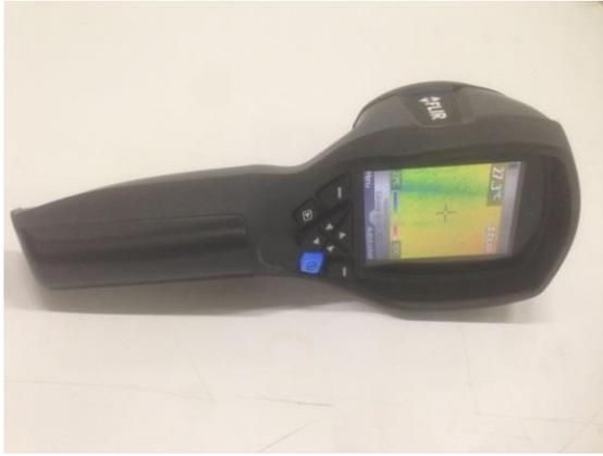
Figure 7. Thermal camera for monitoring the surface temperature of the slabs.
