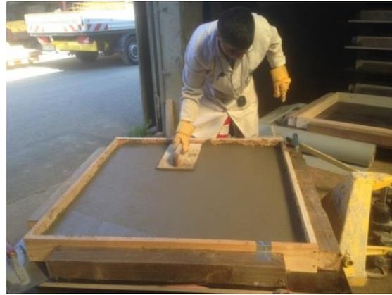
Figure 5. Surface finishing of material.
