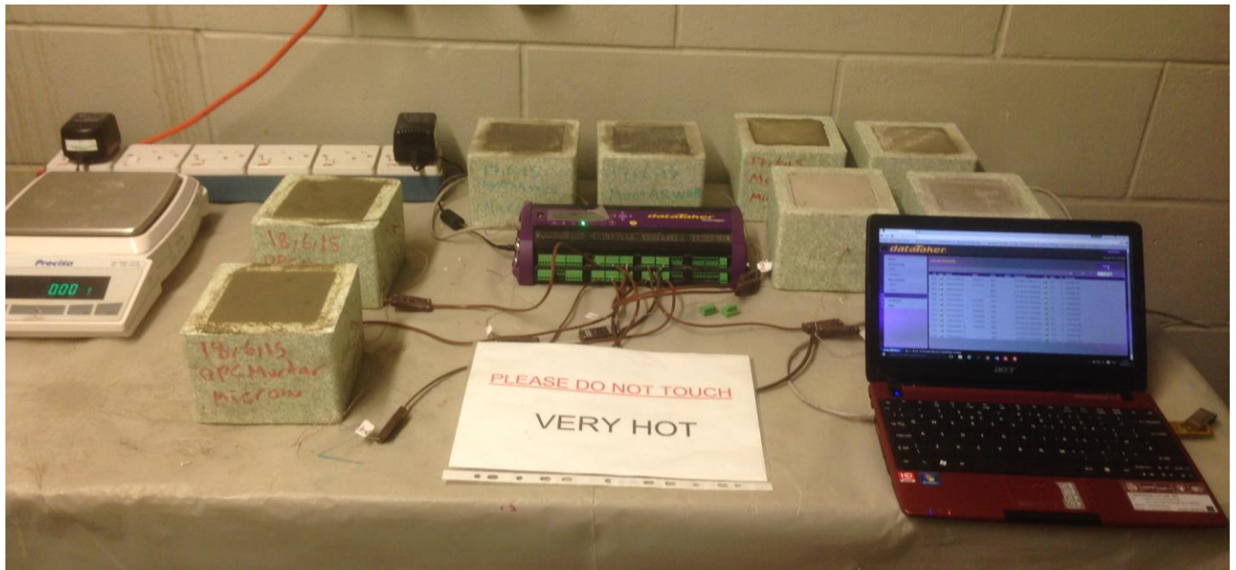
Figure 2. Set up for monitoring internal temperature
