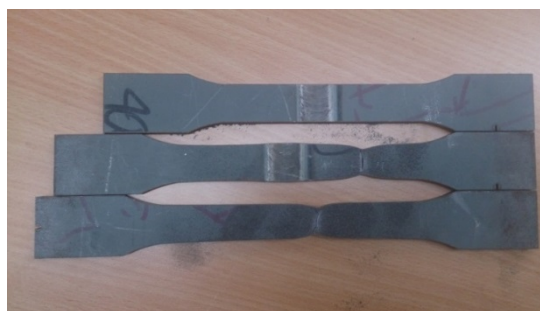
Fig. 14: Photographs of tensile testing samples, the broken FSW sample and also a sample for parent metal.
