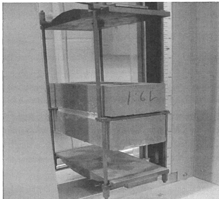
Figure 4 Tensile bond strength test rig
