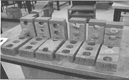
Figure 5 and Figure 6 1:8 lime mortar and 1:8 cement mortar samples
